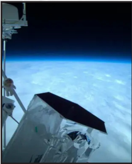
Balloon-borne lidar on PMC-Turbo, a NASA balloon carrying IIAS technology
